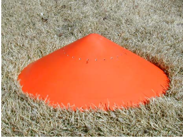
Figure 1. Picture of HITPR. Holes connecting to the diagnostic gauges inside the device are visible.
