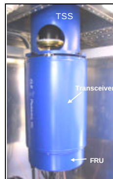
Figure 1 WindTracer® Doppler lidar system configuration showing key subsystems (above). The transceiver cylinder (below) is hung beneath the scanner and measures roughly 40 cm in diameter.
